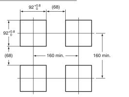
Normal Allowable Deviation= $\pm$ (Value of JIS B 0401-1998 tolerance grade IT18) / 2
