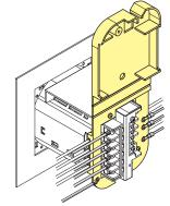
Close the terminal cover and secure it with the screw provided as shown in the diagram below.
