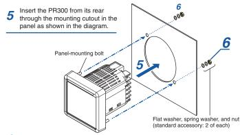
Secure the PR300's panel-mounting bolts by tightening them with the washers and nuts. (recommended tightening torque: 2.0 N•m)
